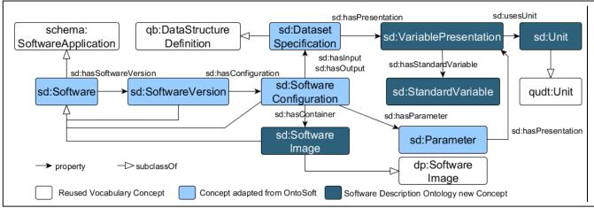
Figure 1: Overview of the main concepts of the Software Description Ontology, used to model OKG-Soft.
