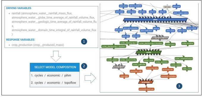
Figure 4: Overview of the process followed by MINT to guide users for model composition. First, users select the driving variables (inputs) and response variables (outputs) to focus on (1). Then, the system looks for available combinations of software models from OKG-Soft (2). Finally, a workflow including all necessary transformations is shown to users (3), highlighting different modeling domains in different colors.
